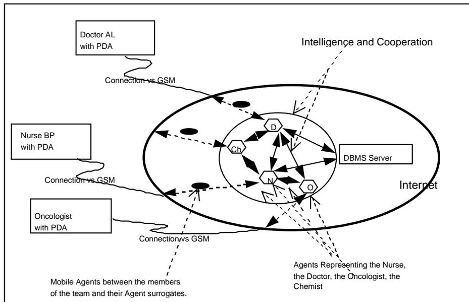
**Figure 3** Schematic of DITIS system infrastructure
