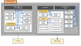
Fig. 3: ENEDI Monitored Sensors and System Probes
