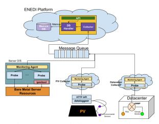
Fig. 2: ENEDI Monitoring System Architecture
