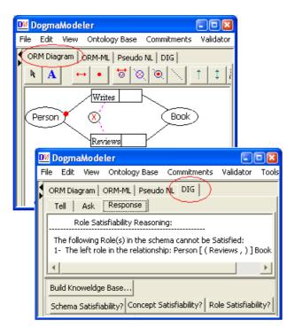
Fig. 18. DogmaModeler's support of description logic-based reasoning.
